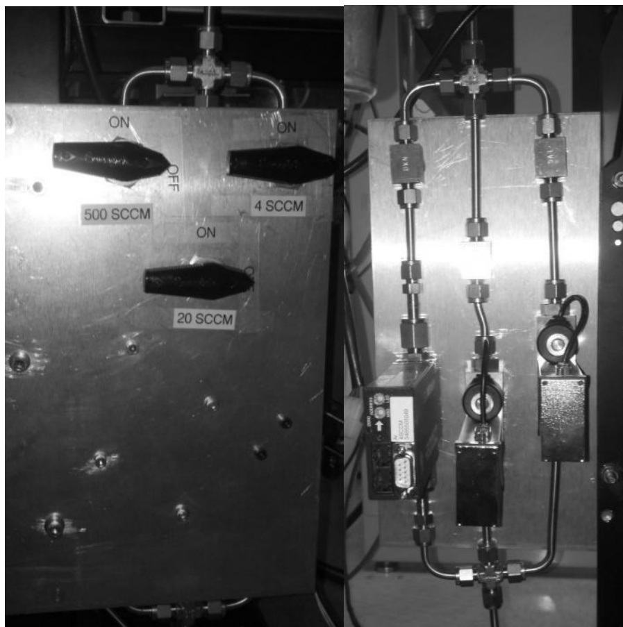
Figure 60: Variable Range Mass Flow Controller Setup: Front View (Left) Back View (Right)
